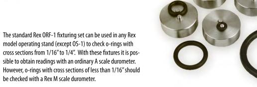
Note: For best results, the fixture should be orientated in the base so that the pins are parallel to the durometer dial face.
